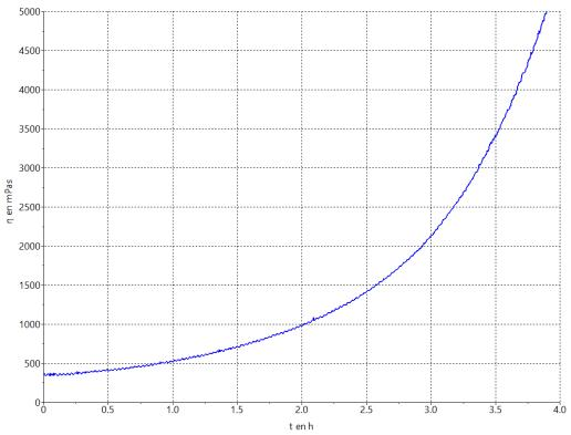
Viscosity measurements realized on rheometer: gap 1 mm, shear rate = 1 s<sup>-1</sup>, ø = 35 mm
