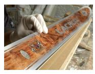
**RESOLTECH 1070 CLEAR** / **1077** is a crystal clear epoxy laminating system formulated to produce clear laminates and high gloss coatings with good mechanical properties while retaining some flex for improved fatigue performance such as for surfboards.
