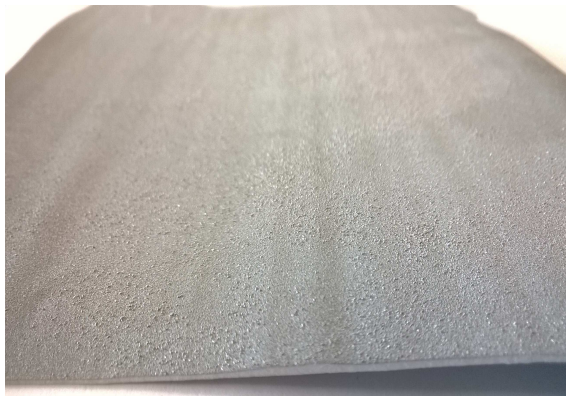
Surface aspect once gelcoat has hardened and the excess of non bonded aluminium particles removed.
