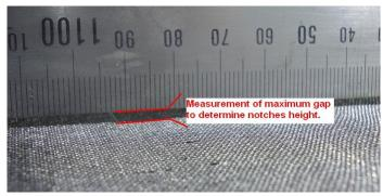
The height of the notches will be defined by the deepest surface unevenness (i.e. slumps of 3 mm on the surface to be bonded will require 5 mm high notches).
