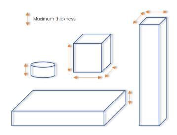
However, thickness is not the only contraining parameter, the quantity cast also influences the exotherm temperature as well as the mold material. See next page.
