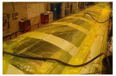
RESOLTECH 1500 / 1504 is an epoxy infusion system with an extremely low viscosity that enables structural composite parts & tools manufacturing with glass of carbon fibre.
