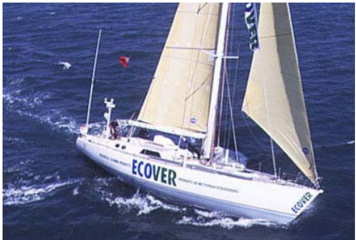
A British Steel Challenge 67' yacht built at Devonport Royal Dockard in 1991. Steel structure faired with the Resoltech epoxy compounds. The yacht sailed around the world against the wind 3 times. Full scale testing from the tropics to Cape Horn.
