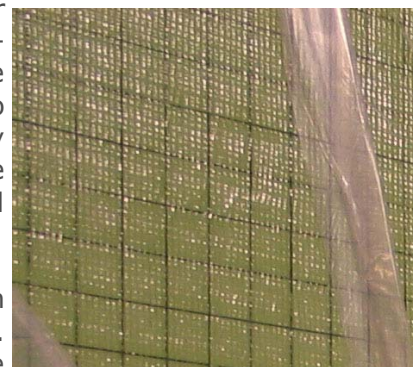
An infused or vacuum bagged composite surface will usually be quite fair. The filler will compensate the fabric overlaps and its texture. A peel ply finish will not require prior sanding.
