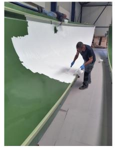
detrimental effect on finish. Once lightly deglazed, surface is ready for a lacquered finish, saving a huge number of coating and sanding hours.
